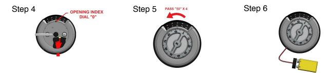
Step 4. Put dial onto dial shaft and slide it into the input until the dial stops. Make sure the dial number "0" is lined up with the center mark (opening index). From the inside of the battery compartment, press in the button fully and hold. Finish installing the dial by pushing the dial in and release the button.
