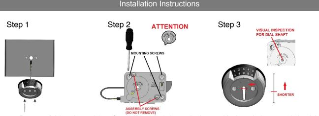
Step 1. Remove dial from keypad (see Step 4 illustration). Insert the input cable through the center hole of the safe door. Using the input mounting screws, mount the input onto the safe door and tighten the screws.
