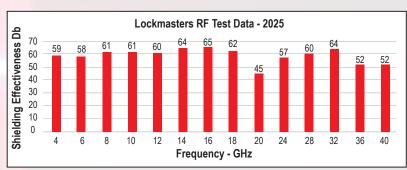
Full STC52 assembly test, independent test facility - January 2025
